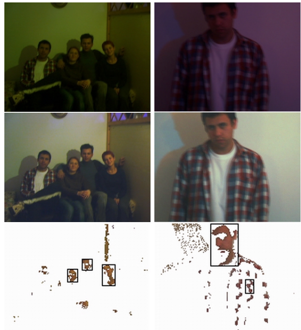
Figure 10: Correlation performance on images from the green (left) and blue (right) subset. On the original image (top) no faces could be detected. After corrected illumination (middle) three faces could be detected on the left image.
