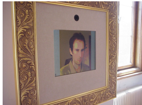
Figure 1: LCD computer monitor dressed up like a precious painting. The round opening above the picture is for the digital camera lens.
