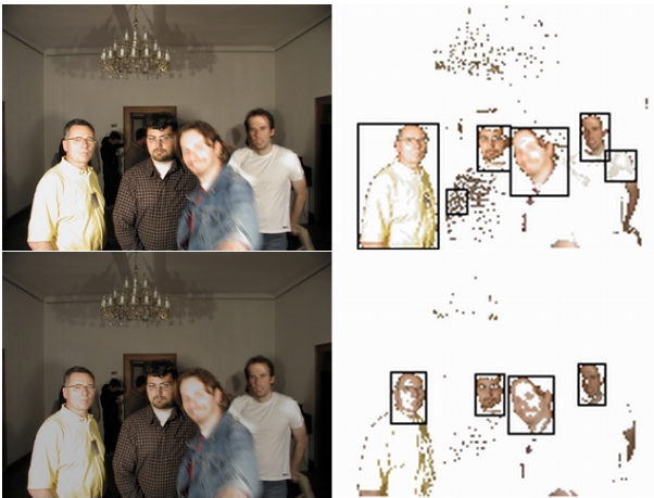
Figure 8: Retinex performance: In the upper part of the figure we see two false detections, while on the lower part this problem was overcome by the Retinex algorithm. The image was taken from the flashlight subset.
