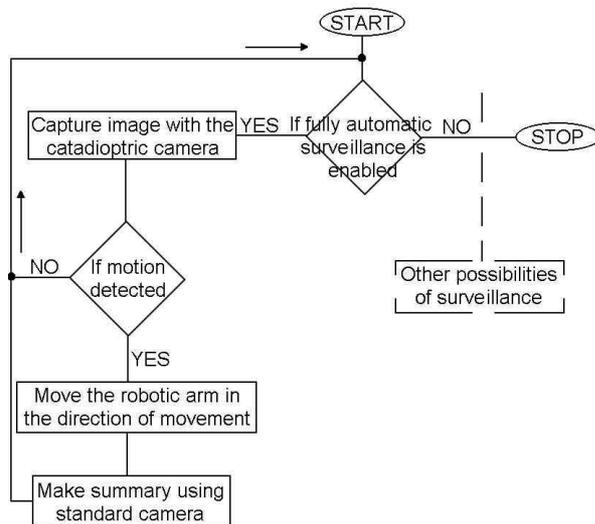
Figure 10. The basic flow chart for fully automatic surveillance in SecurityAgent system.
