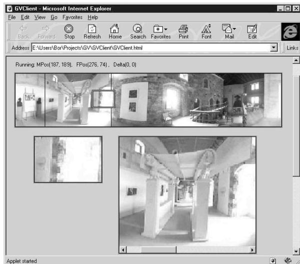
Figure 2. The intuitive GlobalView user interface. The rectangle in the panoramic image indicates the attention window, which presents the current direction of the camera. By moving the rectangle the user controls the direction of the camera. On the bottom of the web page the live video image in actual resolution (left) and a zoomed panoramic view (right) are shown.
