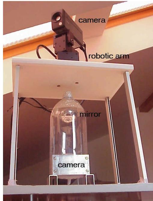
Figure 8. The SecurityAgent basic hardware part combines one standard camera attached on the robotic arm and one catadioptric panoramic camera (it consists of standard camera and spherical mirror), which enables to monitor whole location in every moment.
