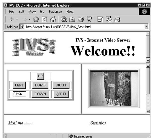
Figure 1. The plain IVS user interface showing buttons for controlling the camera direction.
