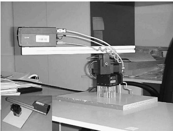
Fig. 2. The system for capturing panoramic depth images.
