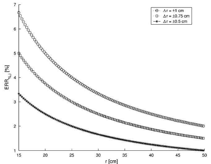
Fig. 3. Sensitivity of the stereo depth reconstructions  $e$  with respect to the changes of parameter  $r$  at different values of  $\Delta r$ .
