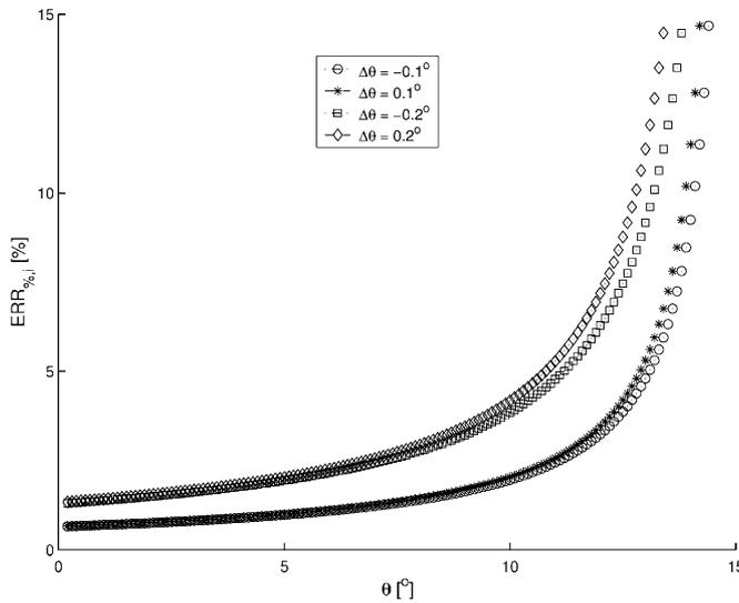
Fig. 4. Sensitivity of the stereo depth reconstructions  $e$  with respect to the changes of parameter  $\theta$  at different values of  $\Delta\theta$ .
