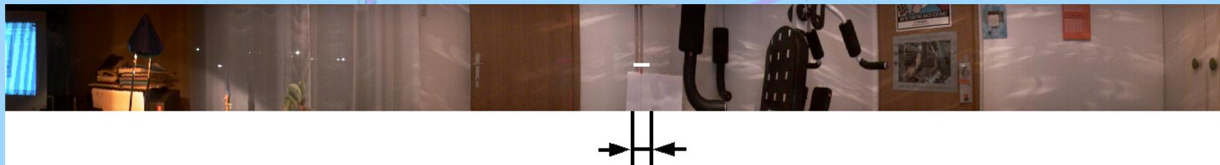
b) constrained length of the epipolar line: 18 pixels,  $2\varphi = 3.6125^\circ$
