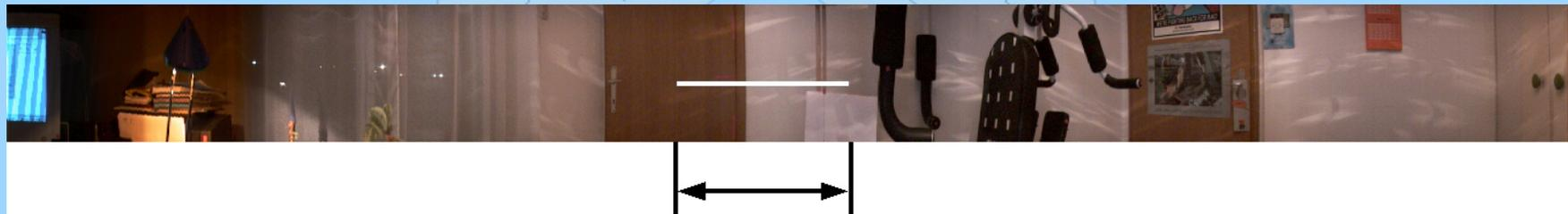
a) constrained length of the epipolar line: 149 pixels,  $2\varphi = 29.9625^\circ$
