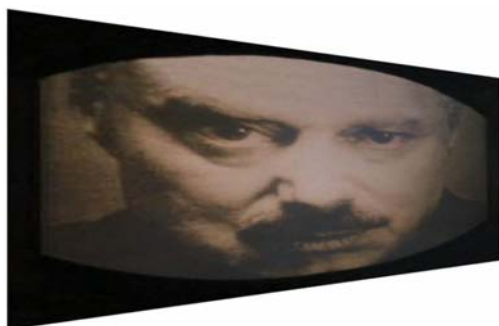
Fig. 6. Transformed frame of a video clip, when the user views it under 30° angle from the right (Big Brother from the film after George Orwell’s novel 1984)
